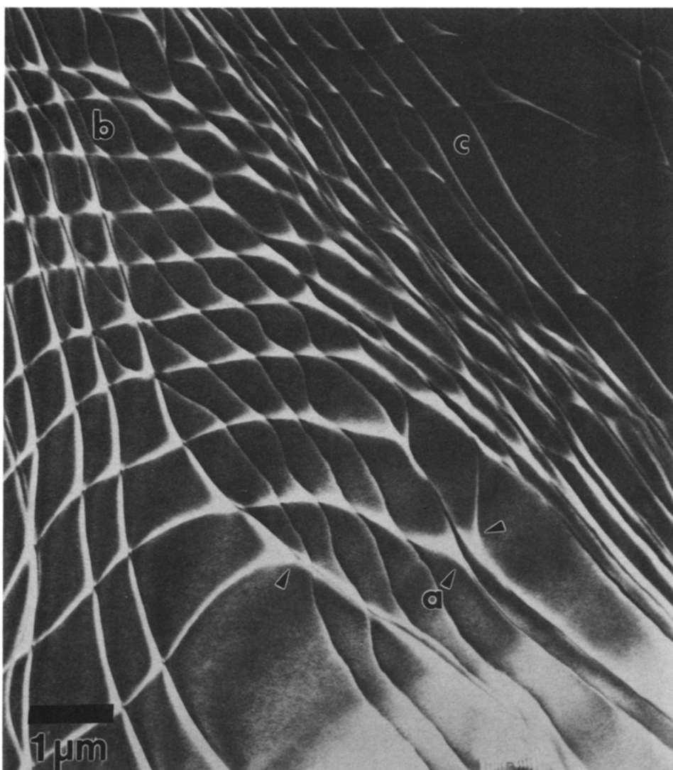
Fig. 9. Dark-field, weak beam, image ( g = 201 ) of extended array of dislocations on parallel (001) planes in sample KP-50. Formation of dipoles is evident at points (arrows) where two or more dislocations merge into a single line. Dislocations within more widely-spaced parallel arrays near a , generally show more curvature when crossed by other dislocations than dislocations in more closely-spaced parallel arrays near area b . Similar behavior is seen in crossing dislocations in area near c .
